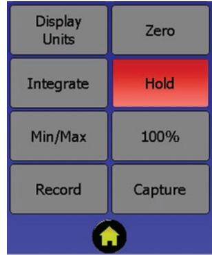
**14B. Zero:** Takes a reading in amps and subtracts that current value from all future readings. Any value below the stored value will be shown as a Zero reading. When measuring small light or current levels, it is a good practice to zero in the environment of the testing and perform period zero validation or re-zero when the conditions in the environment fluctuate (temperature, noise, ambient lighting)
