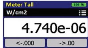
**13B. Display Content:** The content note, located above the display, indicates which display units have been selected by the display units button, followed by the units of calibration and on the far right is the settings access icon.
