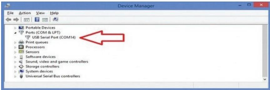
**22A. Setup Procedure:** Allow the computer to assign a com port and install FTDI drivers manually, as needed. Device drivers are located in C, Program Files, International Light Technologies, Datalight III, FTDI folder. To install drivers double click driver CDM.....exe
