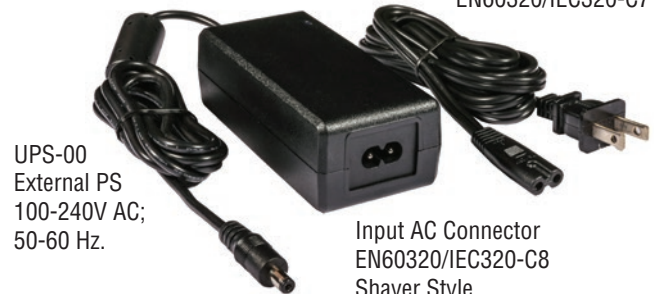
Output DC Connector; Isolated 2.1mm x 5.5mm x 9.5mm; Center Positive
