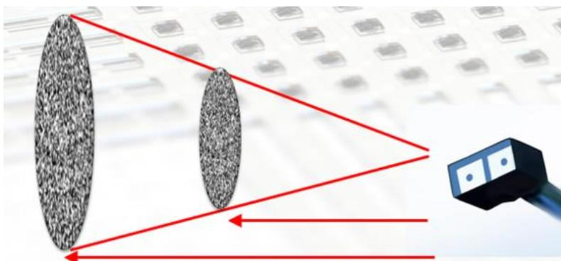
**Figure 5: Principle picture of distance measurement with the NanEye Stereo module and a pseudo random pattern projector**
