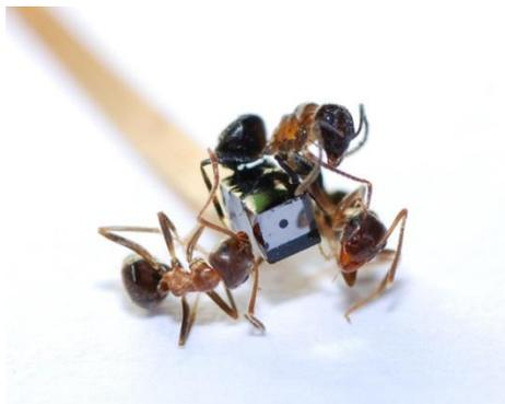
**Figure 1: NanEye 2D 1 mm size camera module**
