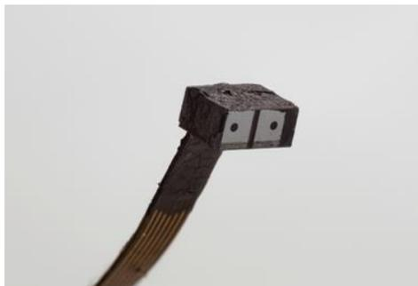
**Figure 4 NanEye Stereo module for 3D vision**
