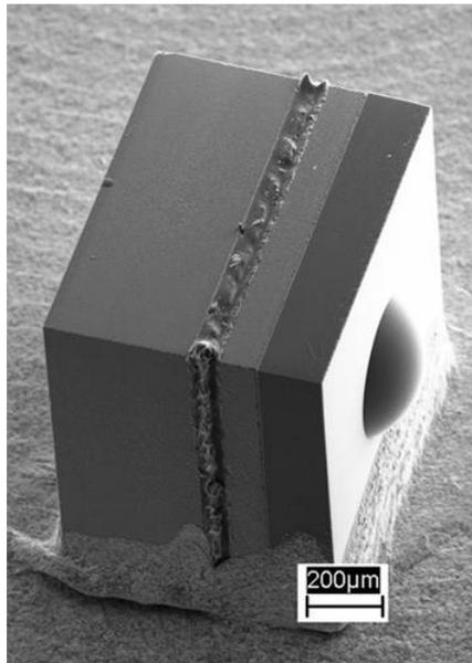
**Figure 2: NanEye 1mm size camera module with wafer level lens in SEM photograph**
