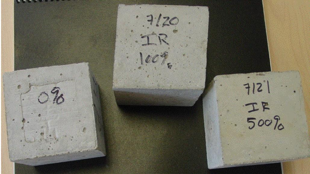
Figure 3. Concrete cubes with known chloride concentrations, prepared at Rutgers, Cubes are 3" on a side.
