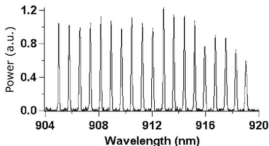
Fig. 3. WBC spectrum of one bar at 35 A.
