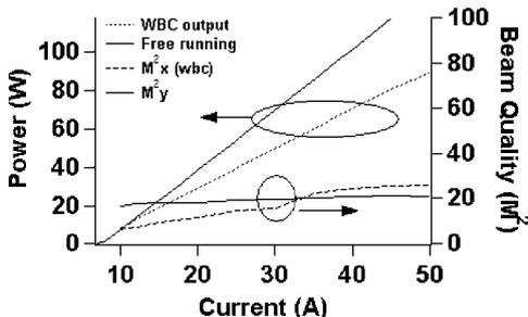
Fig. 4. Left axis, WBC and free-running output power versus current for a three-bar stack. Right axis, beam-combining efficiency and beam quality versus current for a three-bar stack.
