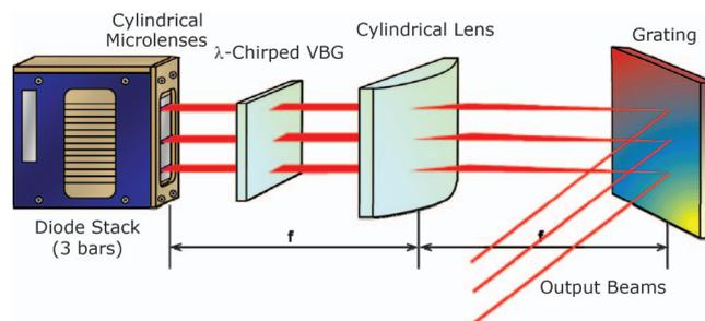
Fig. 1. Basic architecture for WBC of a diode stack (three-bar stack) by using a wavelength-chirped VBG.
