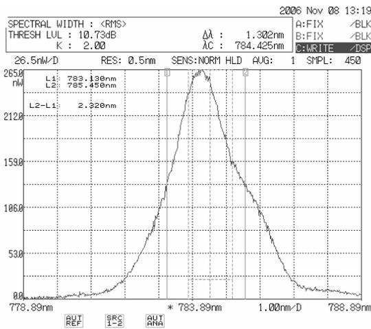
Fig. 7 Stack output without aligned PTC VBG.
